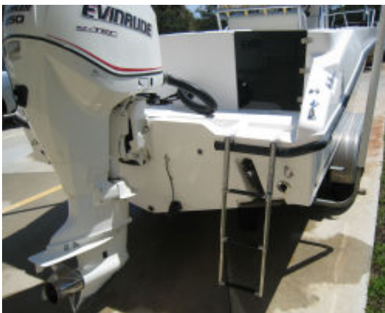
Boarding Ladder and Tuna Door
